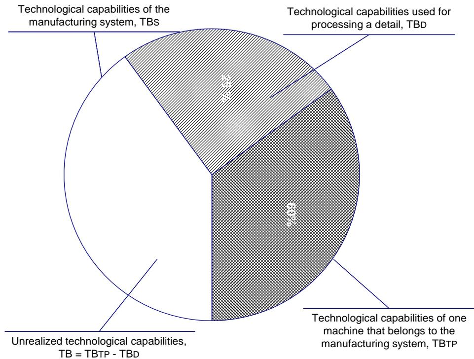
Fig.3. Technological capabilities of the machine tool belonging into technological system and their use
